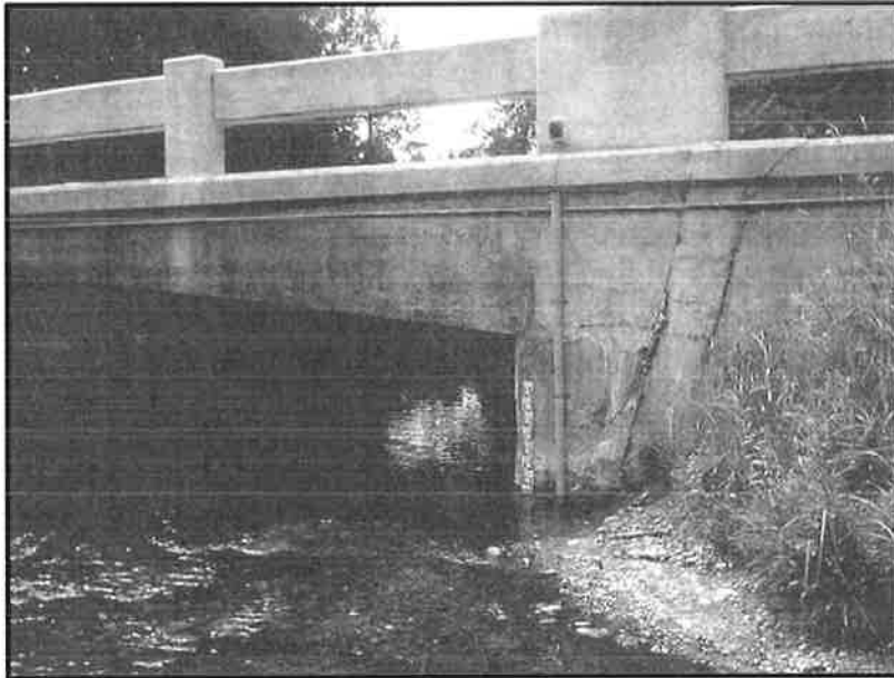
Figure 1. Installation of an AquaSwift water depth unit by Grey Sauble Conservation Authority
