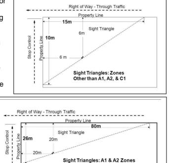
e) In the A1 Zone and A2 Zone a Sight Triangle of 80 metres measured down the Street Line where traffic has the right of way and 26 metres down the other Street Line shall be required. Where both or neither Street Line is a designated right of way, an 80 metres by 26 metres Sight Triangle shall be required along both Street Lines.
